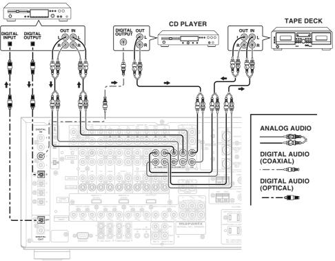
The output audio signal from the TAPE OUT jack and the CD-R/MD OUT jack is the same signal which is currently selected.
